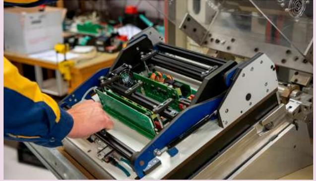
▲ The bare PCB of the UniMulti is placed in its fixture.
